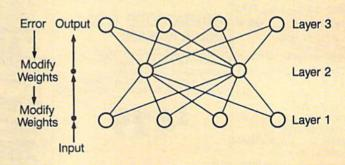
The layout of a back propagation network.
